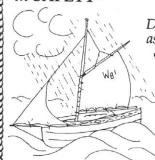
Designed for coastal as well as lake, river & estuary cruising she is particularly sturdy, has reef points on main & jib, built in buoyancy & a self draining cockpit.
